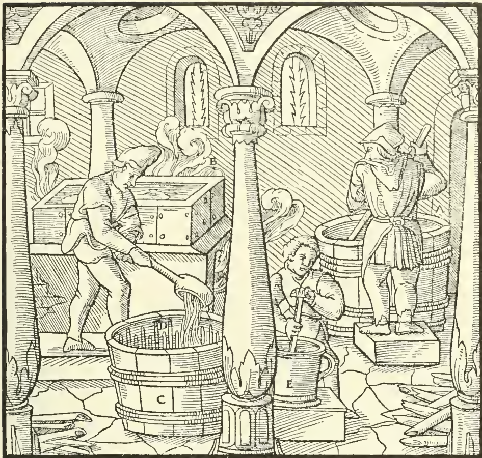
A—VAT IN WHICH THE SODA IS MIXED. B—CALDRON. C—TUB IN WHICH chrysocolle IS CONDENSED. D—COPPER WIRES. E—MORTAR.
